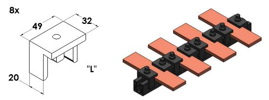
The  $\Omega$  FLAT bar support is a **UNIVERSAL**, **QUICK and CONVENIENT** solution for supporting bars, copper or aluminium. In a flat configuration. It is mainly made of two elements:
