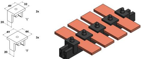
The  $\Omega$  FLAT bar support is a **UNIVERSAL, QUICK and CONVENIENT** solution for supporting bars, copper or aluminium. In a flat configuration. It is mainly made of two elements:
